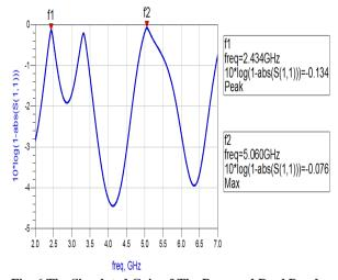
Fig. 6 The Simulated Gain of The Proposed Dual Band Monopole Antenna Designed in ADS
