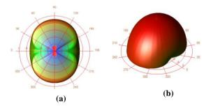
Fig. 9 3-D Radiation Pattern of the Dual-Band Antenna at 2.4 Ghz (a) Bottom View and, (b) Isometric View
