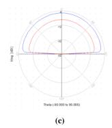
Fig. 8 2-D Radiation Patterns of the Dual-band monopole antenna at 5.1 GHz (a) x-y plane, (b) x-z plane, and (c) y-z plane.
