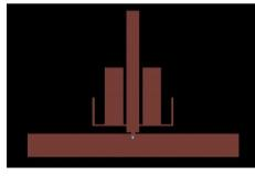
Fig. 2 Proposed Dual Band Monopole Antenna Designed in ADS
