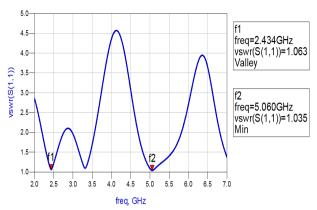
Fig. 5 The Simulated VSWR of The Proposed Dual Band Monopole Antenna Designed In ADS
