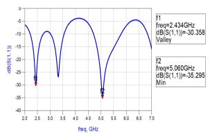
Fig. 4 Return Loss of the Proposed Dual Band Monopole Antenna Designed In ADS
